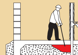
PMT23. Treat around utility pipe.
